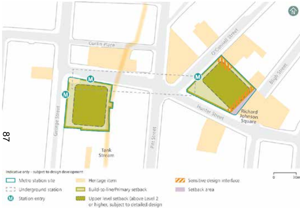
Hunter Street metro - Built form urban design strategies diagram showing proposed setback to Richard Johnson Square Sydney Metro West Environmental Impact Statement
