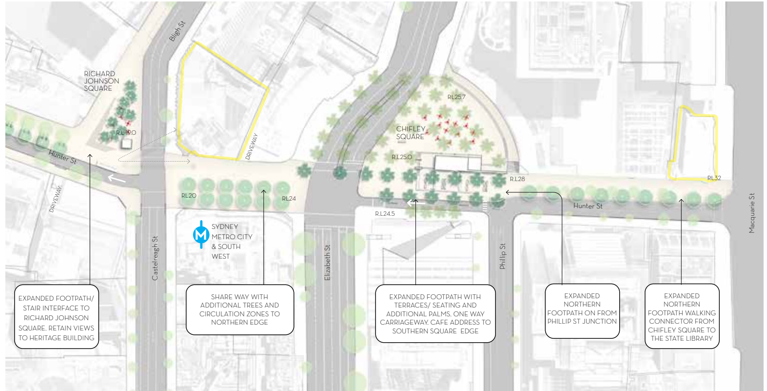
Public domain concept for Hunter Street east of Castlereagh Street (Gallagher Studio Hunter Street Precinct Public Domain Strategy 2022)
