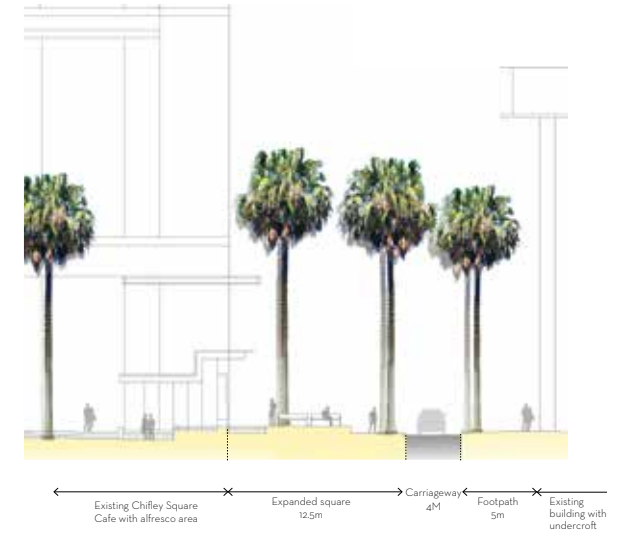
Hunter Street at Chifley Square - sketch concept section (Gallagher Studio Hunter Street Precinct Public Domain Strategy 2022)
